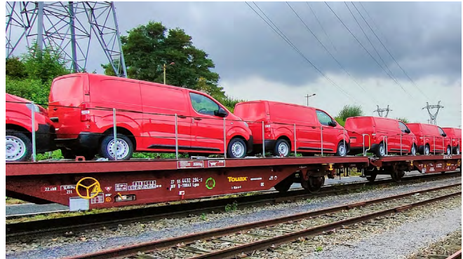
Twin wagons for transport of large vehicles
