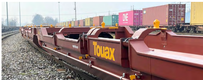
Pocket wagons for transport of semi-trailers
